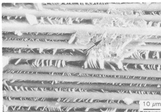
Figure 20 Scanning electron micrograph showing the fracture surface of the Proteus particle-modified composite. The arrow indicates a Proteus particle. The crack propagates from right to left.
