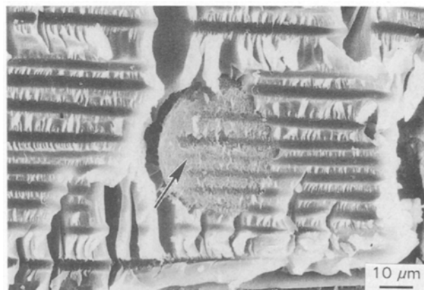
Figure 19 Scanning electron micrograph showing the fracture surface of the Proteus particle-modified composite. The majority of the fracture surface is covered by the epoxy matrix due to the thick layer of the interlaminar resin-rich region. The arrow indicates a Proteus particle. The crack propagates from right to left.
